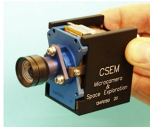
Weighing 100 grams each, the cameras compose part of CIVA (Comet nucleus Infrared and Visible Analyzer), one of ten on-board instruments for Philae's in situ analysis of the comet.
