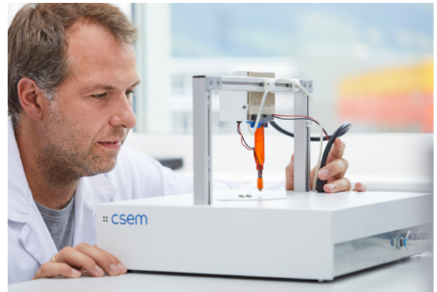
Pneumatic head with integrated air flowrate sensor and micro-valve
