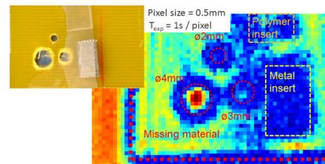
Figure 2: (left) image of glass fibre composite plate; (right) THz image.
