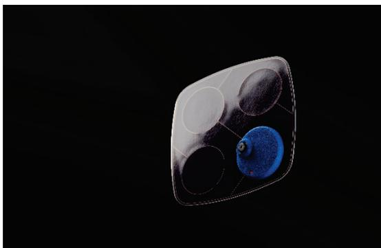
*Witness prototype measures 80 mm by 80 mm; The diameter of the camera button is 30 mm, its thickness 4 mm.*
