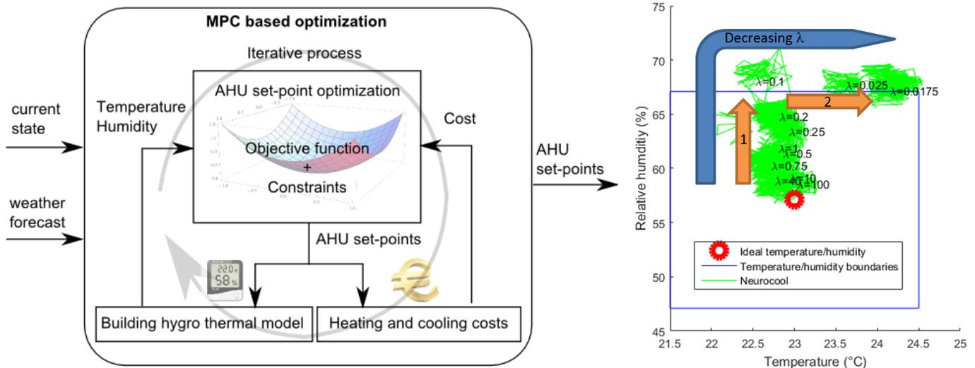
MPC based HVAC control overview (left) measured indoor temperature/humidity for various comfort ( $\lambda$ ) settings (right).
