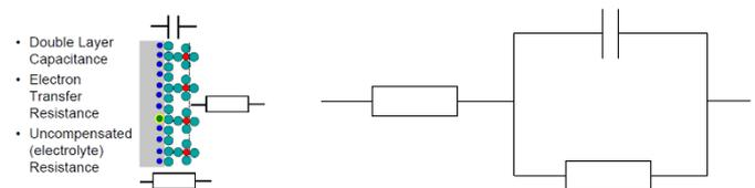
Such a circuit (Randles circuit) is valid for high-frequency ranges, where mass transport effects are minimal.
