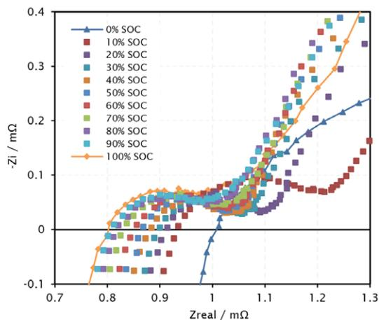
The measurements were obtained between 0.01 and 3000 Hz at 0.1 A using a "Gamry Reference 3000" EIS test equipment. The Nyquist plot clearly shows the dependence of the electrolyte or solution resistance ( $Z_{real}$  at zero  $Z_i$ ) and the semicircle range on the SOC of the cell. Lower impedance values are found at higher SOC levels. The plot also differs from the one measured with the new cell, i.e. at zero cycles.
