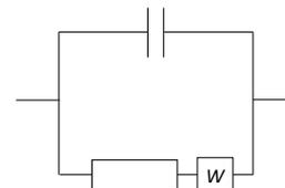
In general, electrolyte, insulating layer (SEI) and charge transfer resistance are dominant at high frequency and diffusion or mass-transfer resistance becomes significant at low frequencies.
