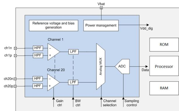
Figure 1: A simple system-on-chip (SoC) with different components.
