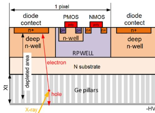
Figure 1: Lateral view of the pixel.
