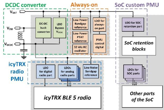
Figure 1: Block diagram of the integrated icyTRX with PMU.
