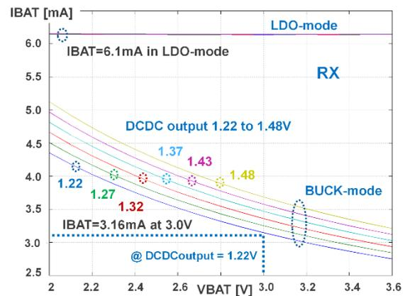
Figure 2: RX current consumption versus supply voltage.
