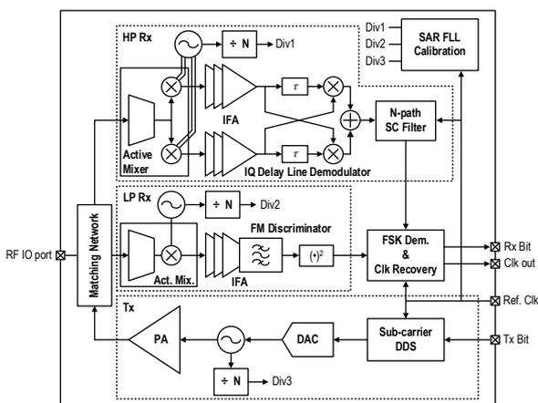
Figure 1: FM-UWB transceiver block diagram.
