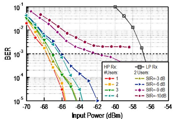
Figure 2: BER curves for the two receivers.
