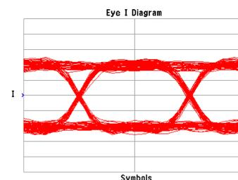
Figure 2: Eye-diagram with pre-distortion filter applied.
