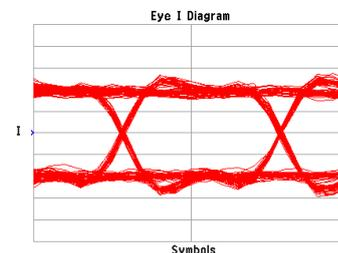
Figure 1: Eye-diagram without pre-distortion filter applied.
