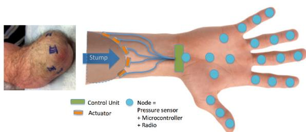
Figure 1: Schema of WiseSkin. A WSN embedded in a polymer senses the pressure over the skin, transmits the data via wireless multi-hop network to a CU, which transfers the stimuli to the nervous system of the user (source of the stump image: Lund University).
