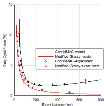
Figure 2: Duty cycle as a function of Latency. The Modified-Glossy protocol displays a lower duty-cycle in the entire range of latencies.
