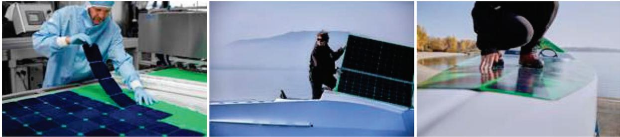
*Specially made solar modules have been developed by CSEM for the Arctic Solar by Icade expedition. Designed to resist to the extreme conditions of the voyage, they enable Anne Quéméré to move about in her vessel.*
