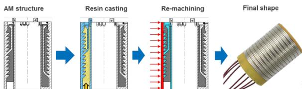
Figure 1: New process with additive manufactured parts (patent pending).
