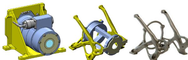
Figure 3: Example of topology optimization made at CSEM.
