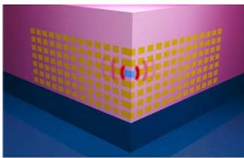
Figure 1: Schematic of one quarter model of the 3D acoustic cage with the mechanical resonator.
