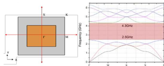
Figure 2: Unit cell and band structure indicating bandgap: frequency vs reduced wave vector path  $\Gamma$ -M-K-X- $\Gamma$ .
