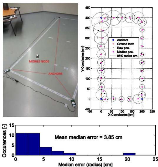
Figure 1: 2D indoor localization setup (left), raw results (right) and histogram of median position error for 10 measurements per position.
