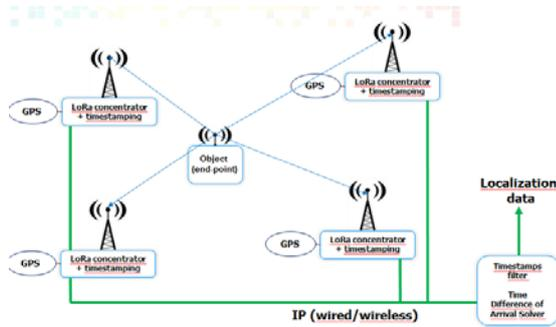
Figure 1: Typical LoRa infrastructure for localization.
