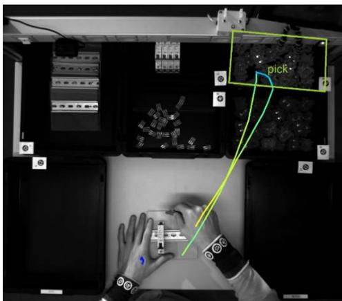
Figure 1: System-camera view. A picking action is recognized.
