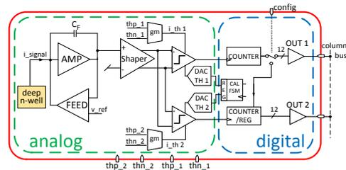
Figure 2. Building blocks of the single pixel.
