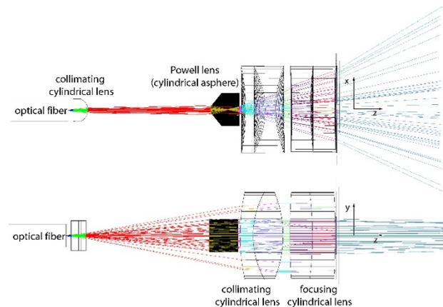
*Figure 1: Scheme of the laser line-generator optics. The upper image illustrates the "line-spreading-beam-path" as a scheme in the xz-plane, the lower image shows the "line-focusing-beam-path" as a scheme in the yz-plane.*
