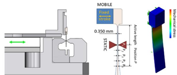
Figure 3: Alternate bending fatigue test principle.
