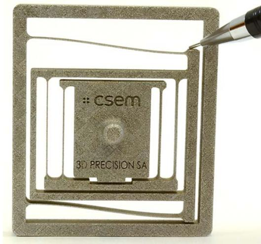
Figure 1: 316L stainless steel AM-SLM built linear stage.
