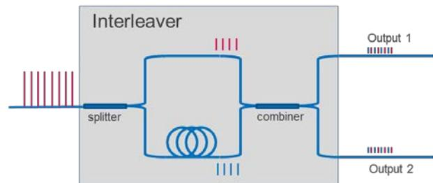
Figure 2: 1-stage optical pulse interleaver scheme resulting in duplication of pulse repetition rate.
