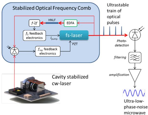
Figure 1: System diagram for photonics-based source of ultra-low phase-noise microwaves.
