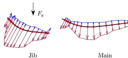
Figure 3: Visualization example of pressure distribution based on wind tunnel measurements at an apparent wind angle of 20°.
