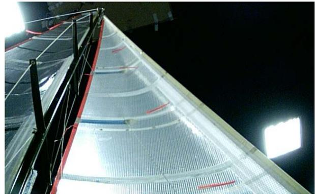
Figure 2: Pressure-strips (in white) applied to the main sail of the 1:10 scale model during wind tunnel test.
