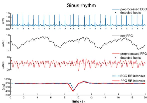
Figure 1: Example of ECG and PPG signals and post-processing results during SR.
