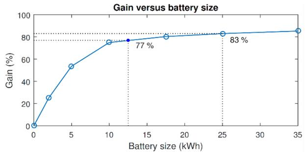
Figure 2: Optimization gain vs. battery size. When the battery size is halved from 25 to 12.5 kWh, the gain is reduced by only 6%.
