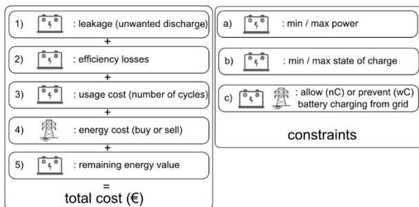
Figure 1: The different terms of the objective functions and constraints that are taken into account in the optimization problem.
