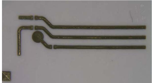
Figure 3: Printed electronic features on nanoporous paper.
