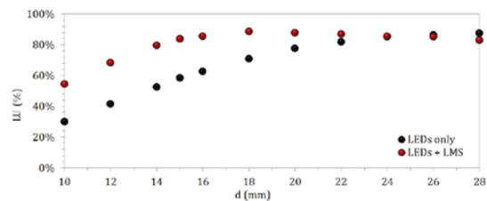
Figure 3: Luminance uniformity of a 15 mm thick  $600 \times 600 \text{ mm}^2$  area lighting module as a function of the air gap thickness.  $t$ : 1 mm, LED pitch: 30 mm.
