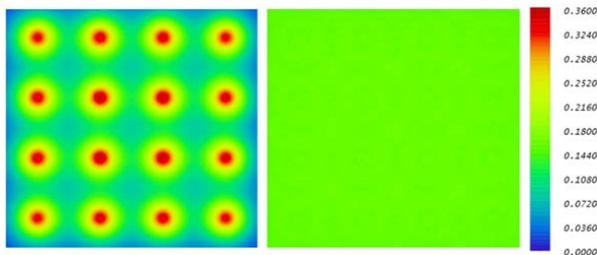
Figure 1: (Top) Lambertian (red), cosine-cubed (dotted red) and optimum batwing (solid red) normalized intensity distributions. (Bottom) Irradiance produced by a  $4 \times 4$  LED array over a plane target situated 15 mm above the array for Lambertian (left) and batwing-shaped (right) LEDs.
