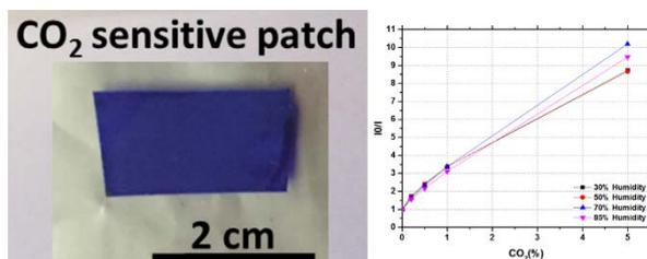
Figure 1: (Left) Picture of CO<sub>2</sub> sensing patches; (Right) Stern-Volmer curves of CO<sub>2</sub> sensitivity showing the low impact of humidity.
