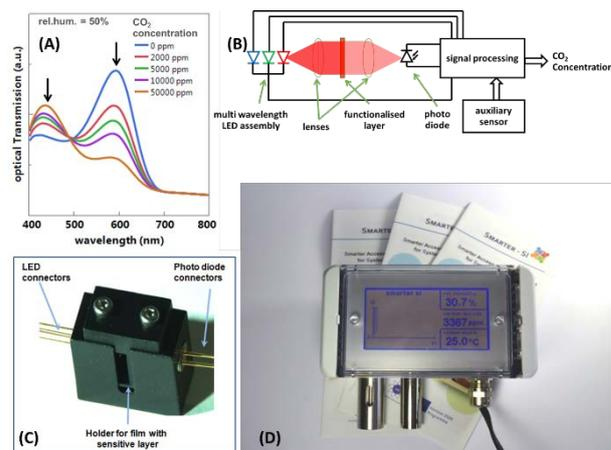
Figure 2: (A) Absorbance spectra of *m*-cresol purple dye functionalized sensitive patches at different CO<sub>2</sub> concentrations; (B) Working scheme of the optical reader; (C) picture of the reading module; (D) Picture of the sensor demonstrator for indoor air quality monitoring.
