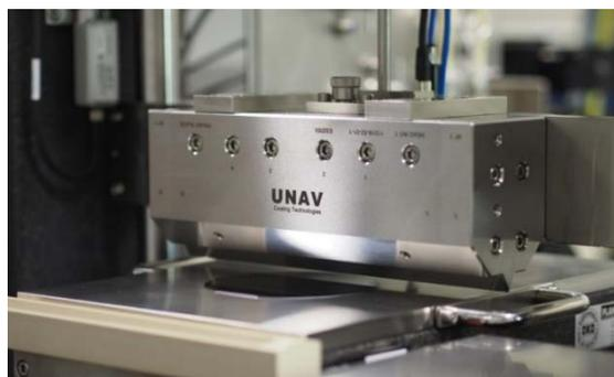
Figure 1: photograph of a slot die deposition head.
