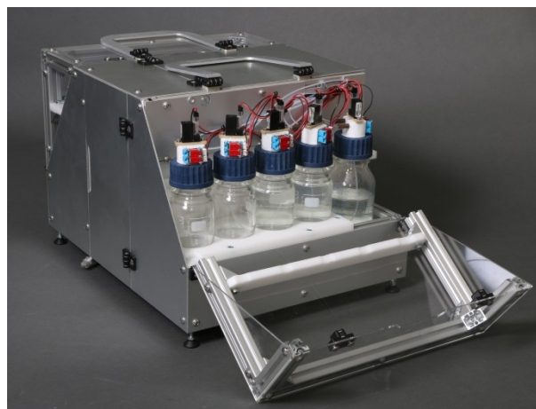
Figure 2: Food quality monitoring system integrating a controlled, pressure driven dispensing subsystem (all five bottles are controlled).
