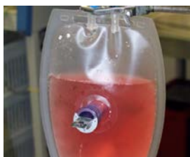
Figure 2: Biosensor integrated in a single use bioreactor [2].
