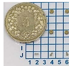
Figure 3: Laser micro-machining of coated silicon wafer and of Nanofoil metal sheet into small shape preforms.
