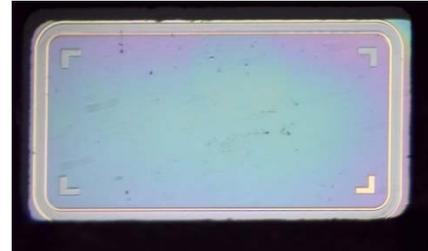
Figure 2: Hermetically sealed glass on silicon package.
