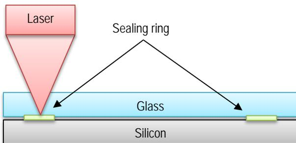
Figure 1: Laser-assisted sealing of glass lid on silicon with sealing ring.
