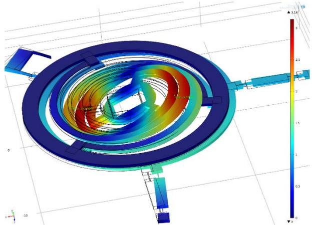
Figure 2: The deformation of the silicon mechanism that converts a linear actuation in a tilting movement of the mirror.
