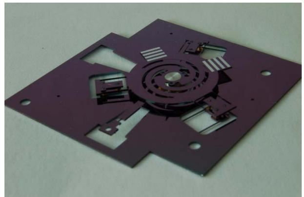
Figure 3: Functional model assembled from precision silicon mechanical parts.
