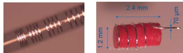
Figure 3: 3D printed antennas.
