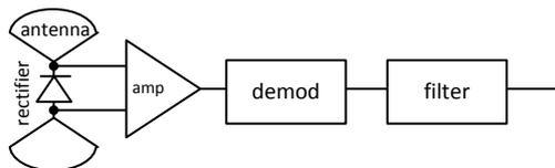
Figure 1: Detector architecture.
