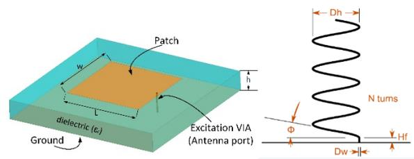
Figure 2: Patch antenna (left) and helix antenna (right).
