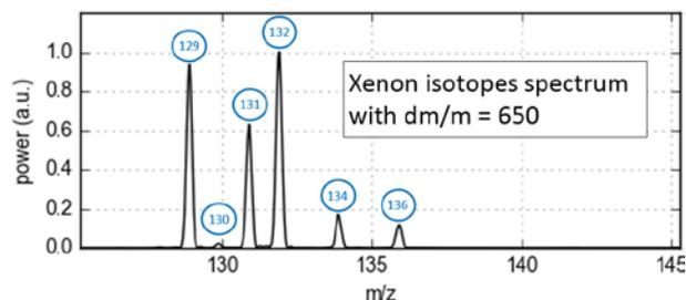
Figure 3: Measurement of Xenon, displaying the natural isotopes.
