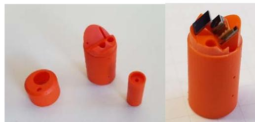
Figure 4: Endoscope head prototype.
