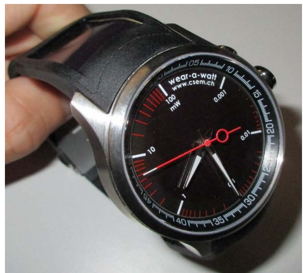
Figure 2: Wearable prototype with thin-film PV cells integrated in the wristband (2016). The cells are put on both parts of the plastic wristband and cover an area of 2.0 × 4.5 cm 2 . From indoor to outdoor the light intensity typically varies typically by 3 orders of magnitude which is why the milliwatt units are represented on a logarithmic scale on the watch dial (white and red tick marks) instead of the usual hour ticks.
