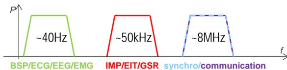
Figure 2: Frequency band for BSP, IMP and communication.
