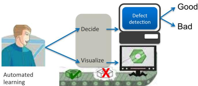
(Semi-) Automated quality control. An operator can choose the option to visualize the images and make the decision of conformity (semi-automated), or let the system make the decision (automated).
