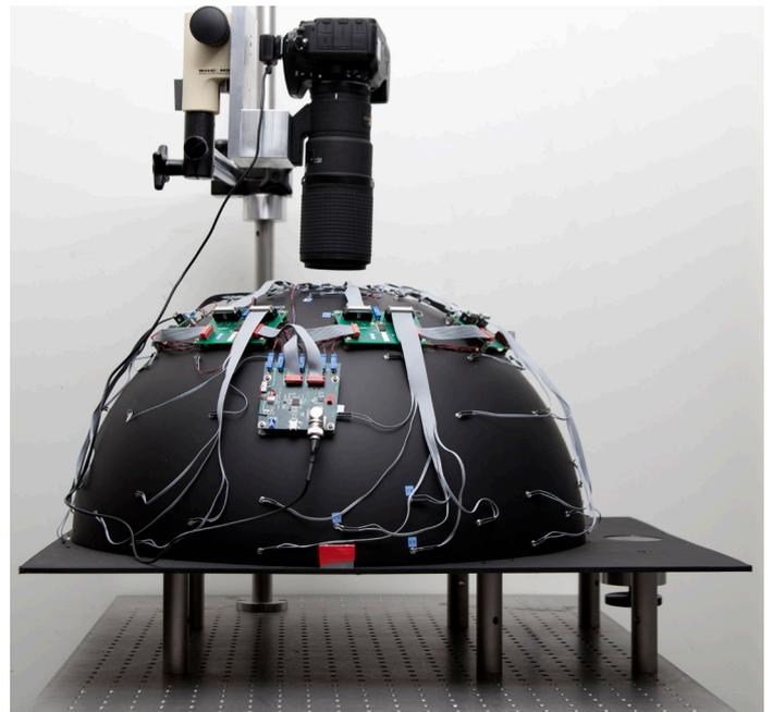
EagleEye hemisphere. The LEDs in this setup are at different elevations and azimuths, while the camera looks at the samples from the top.
