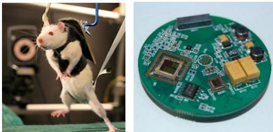
Figure 2: Left: rat walking with electrical stimulations on spinal cord (EPFL [1]). Right: First version of PCB for neuro-prosthesis.
