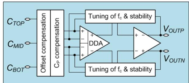
Figure 2: Simplified block-schematic of the fully differential C2V.
