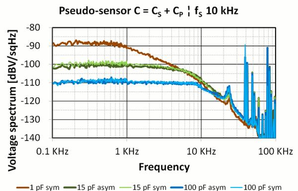
Figure 3: Noise measurement of the C2V with pseudo-sensors.
