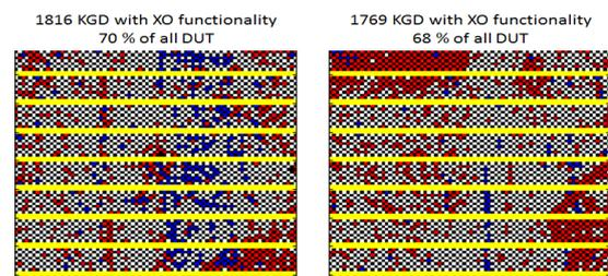
Figure 2: Wafer map showing timing module manufacturing yield.
