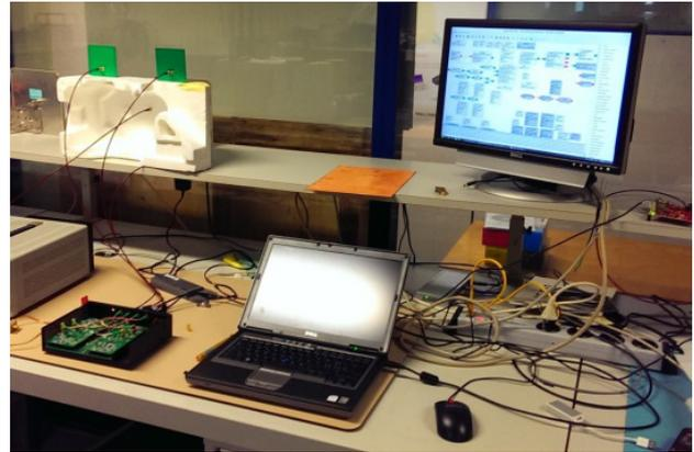
Figure 1: Setup for test and demonstration of motion sensing behind obstacles using and SDR platform and MIMO principles.
