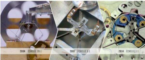
Figure 1: The Genesis of the Genequand regulator. From the 20:1 wood scale model (left) to the 1:1 silicon based prototype (right).
