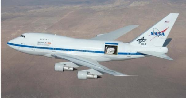
Figure 1: SOFIA Boeing 747 with the telescope door opened.
