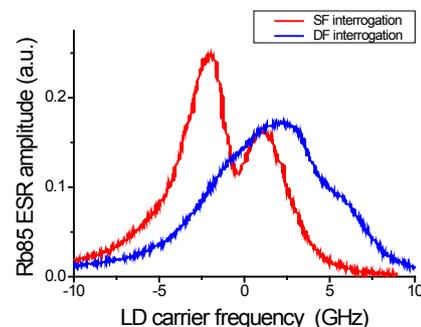
Figure 3: ESR in <sup>85</sup>Rb atoms at 145 kHz ( $B_z=31\mu\text{T}$ ) vs carrier optical frequency under SF (red curve) and DF (blue curve) interrogation.
