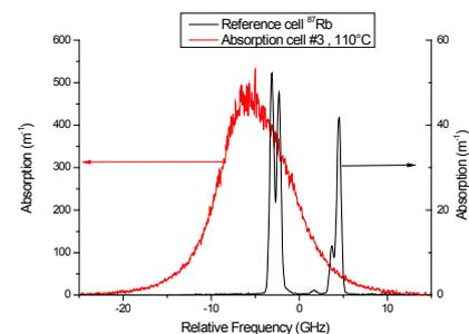
Figure 1: Measured absorption spectra of representative Rb-Xe-N<sub>2</sub> cell at 110°C (red curve) and of the reference cell with <sup>87</sup>Rb and no buffer (black curve).
