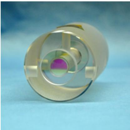
Figure 1: Optical reference cavity implemented at CSEM.
