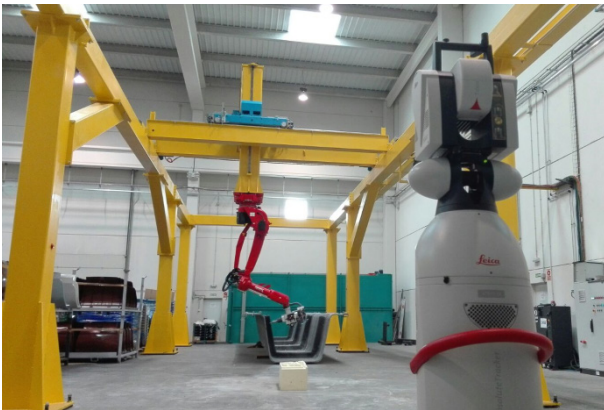
Figure 1: The Megarob prototype with overhead crane, robot arm, and laser tracker.
