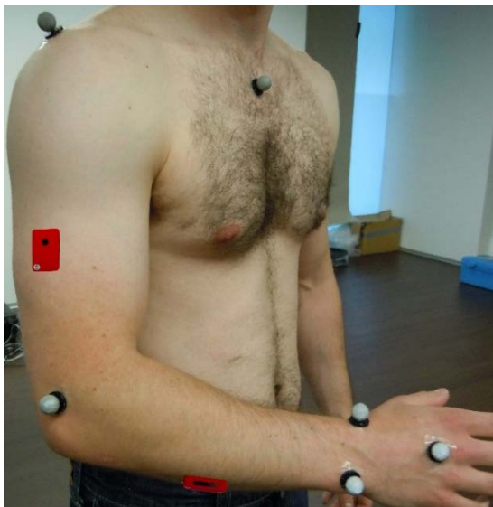
Figure 2: Subject with mounted reflectors (silver) and IMUs (red).
